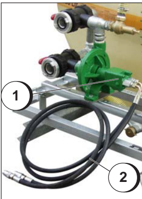
Figure 5.2.2a: Hydraulic motor (1) and hoses (2)
