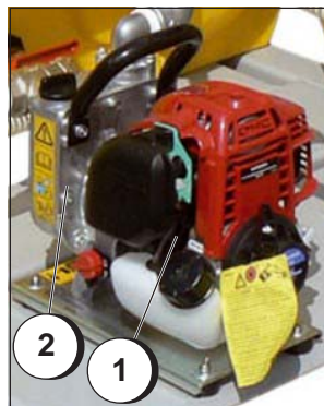
Figure 5.2.1b: - Petrol engine (1) - Pump 130l/min (2)
