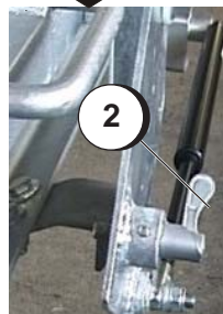
Figure 5.5.2e: Swivelling lever back turned to lock position
