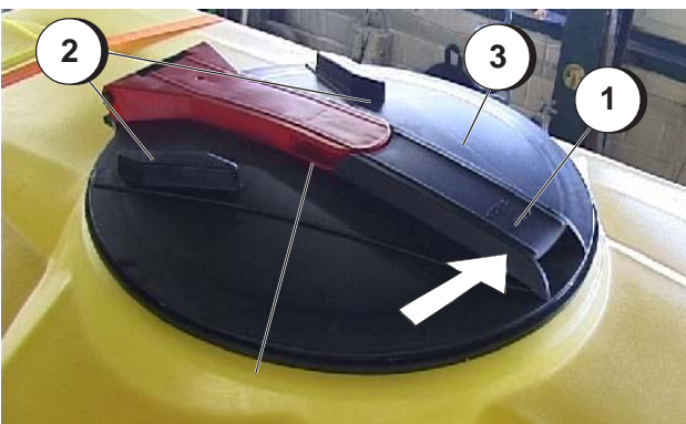
Image 5.4.2b: couvercle rabattable (cuve PE)
