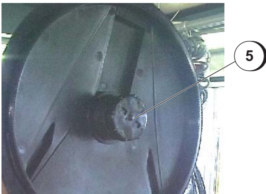
Figure 5.4.4 BWS 130: Float as baffle (view of lid bottom)
